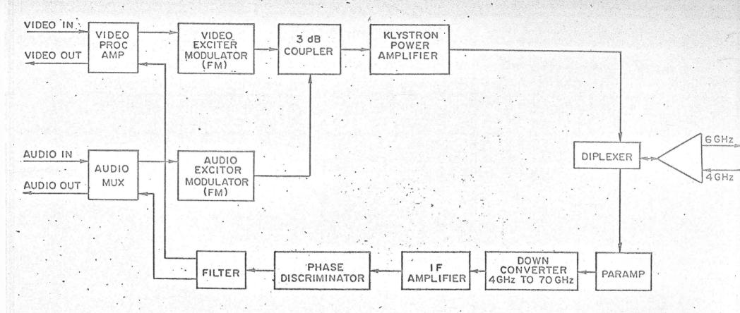
Figure II Block Diagram of Ground Station for Two-way Audio and Facsimile Channel
