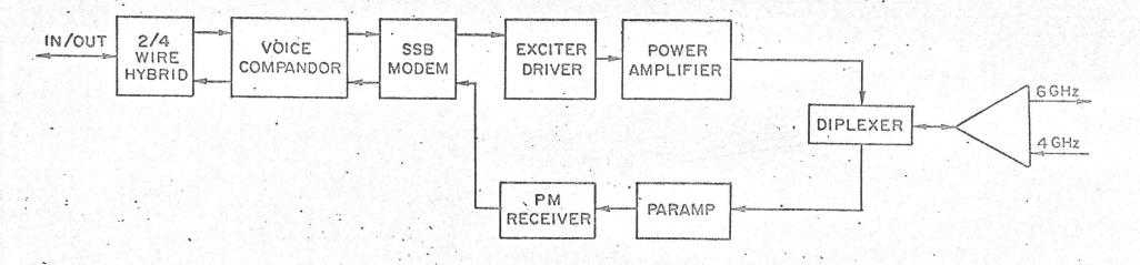
Figure I Block Diagram of Ground Station for Two-way Voice Channel
