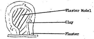
The clay is then removed and the model cleaned and the space previously occupied by clay filled with gelatine (or P.V.C.).
