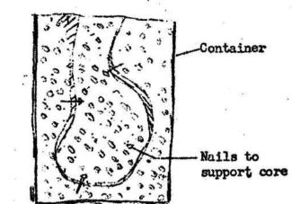
Place in suitable container and pour investment mixture Vibrate to romove air pockets
